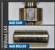
The lack of lubricity in ULSD is the main factor in the catastrophic failures of the CP4 Fuel pumps. High rates of wear introduce metal shavings into the fuel system, creating wear that damages your injectors, cylinder walls, pistons and rings costing several thousands of dollars to repair.
