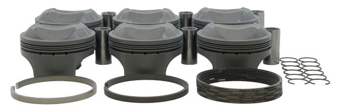
The pistons are machined from forgings with narrower and shorter skirts to reduce weight and friction. They are then dual coated, with phosphate and MAHLE's proprietary GRAFAL® skirt coating. The phosphate is a dry film lubricant designed to help protect the pin bores from galling and ring grooves from micro-welding. The GRAFAL® anti-friction skirt coating is designed to reduce drag, wear and noise.
